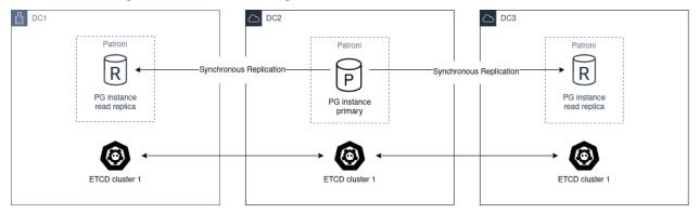
We must deploy a cluster of etcd, ZooKeeper or Consul through the different DC, with a minimum of 3 nodes, one in each zone.
