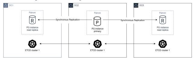
We must deploy a cluster of etcd, ZooKeeper or Consul through the different DC, with a minimum of 3 nodes, one in each zone.
