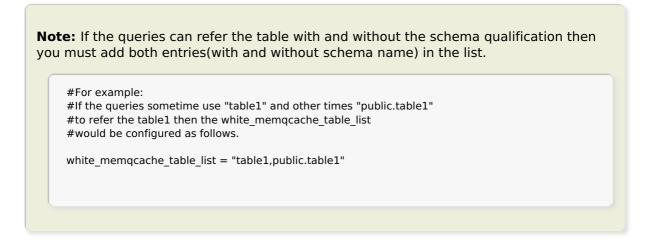
This parameter can be changed by reloading the Pgpool-II configurations.
