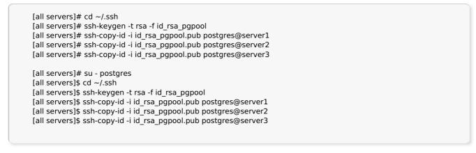
After setting, use ssh postgres@serverX -i ~/.ssh/id\_rsa\_pgpool command to make sure that you can log in without entering a password. Edit /etc/ssh/sshd\_config if necessary and restart sshd.
