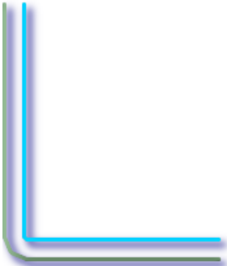
15, 'quad_segs=4 join=bevel' shown with original line
