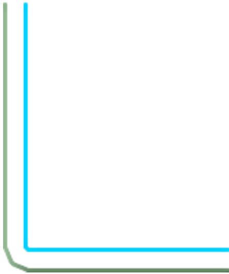
15, 'quad_segs=4 join=bevel' shown with original line
