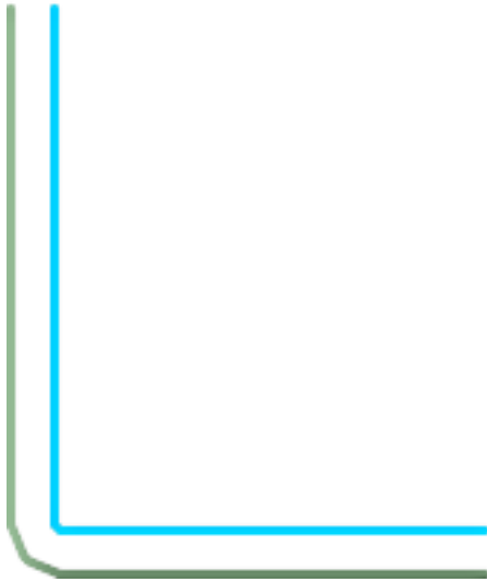
15, 'quad_segs=4 join=bevel' shown with original line
