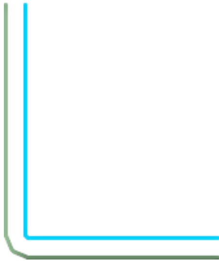
15, 'quad_segs=4 join=bevel' shown with original line
