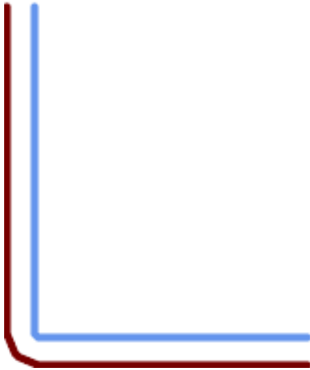
15, 'quad_segs=4 join=bevel' shown with original line
