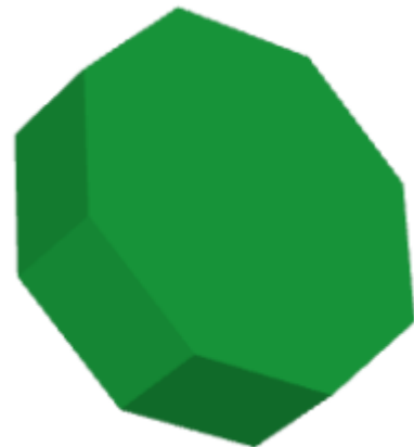
Hexagon extruded 30 units along Z produces a PolyhedralSurfaceZ
