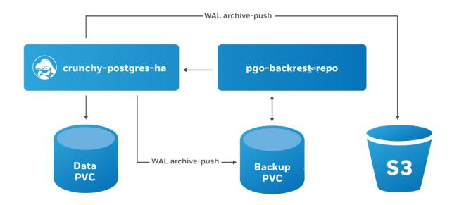
The PostgreSQL Operator leverages a pgBackRest repository to facilitate the usage of the pgBackRest features in a PostgreSQL cluster. When a new PostgreSQL cluster is created, it simultaneously creates a pgBackRest repository.
