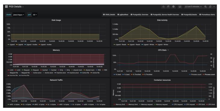
Pod details provide information about a given Pod or Pods that are being used by a PostgreSQL cluster. These are similar to "operating system" or "node" metrics, with the differences that these are looking at resource utilization by a container, not the entire node.
